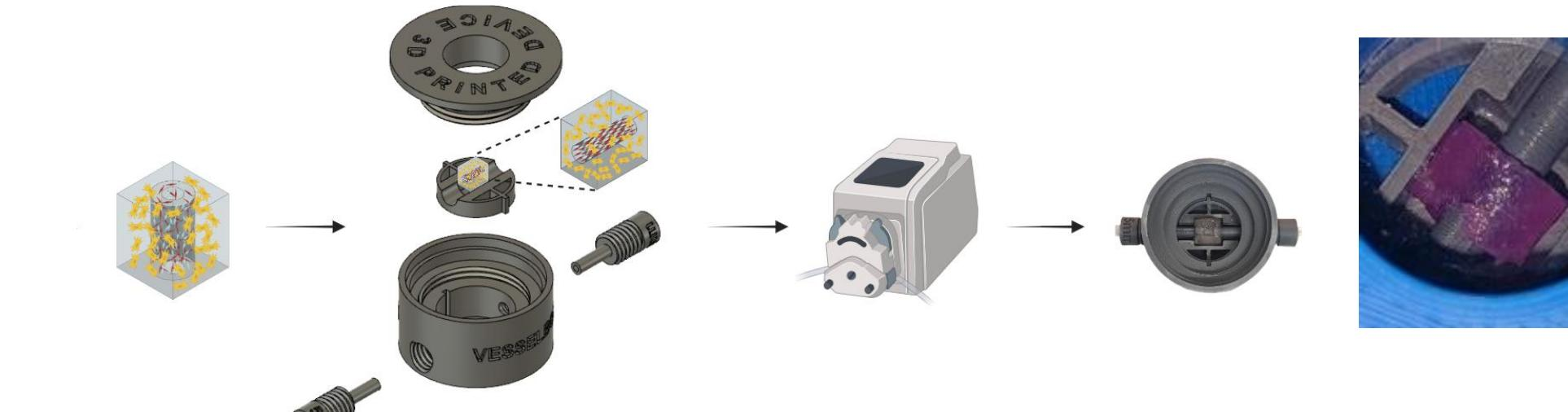
After 14 days of static maturation, the vascularized scaffolds are perfused in the VesselBox device connected to a peristaltic pump. The adapters ensure that medium only passes through the inner hole of the scaffold, guaranteeing a selective perfusion.
