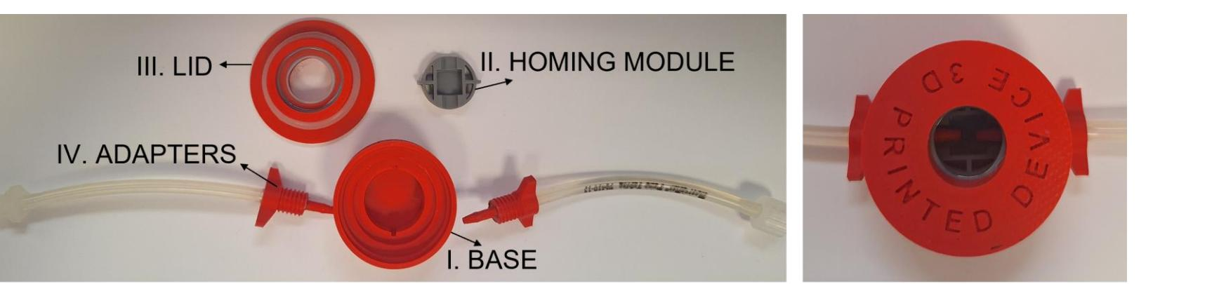
VesselBox includes: I. a base II. a homing module to allocate the scaffold III. a lid with optical window IV. two adapters to selectively perfuse hollow scaffolds in a sterile and sealed environment. The VesselBox is 3D printed with autoclavable materials.
